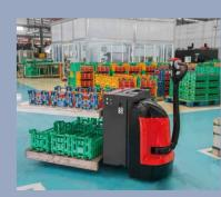
The support arm lift capacity is 2000 kg while the mast lift capacity is 800 kg
