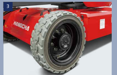
Tires: foam-filled tires with good off-road performance
