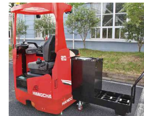
Standard configuration: Battery side roll-out + trolley(optional)
